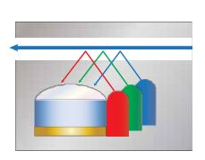
The light from 3 RGB color LED (red, green and blue) used as a light source is reflected by the document. This light is received in turn by the CIS sensor, which performs the actual scan
